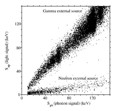
Figure 8.2. Discrimination capability of the CRESST test detector.
