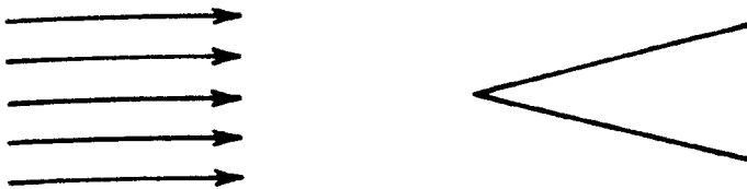
Fig. 6.2. Air current blowing against the edge of a wedge, viewed in cross-section
