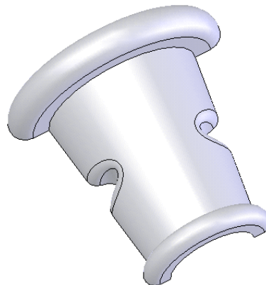
Figure 15-105 Resultant fillet feature
